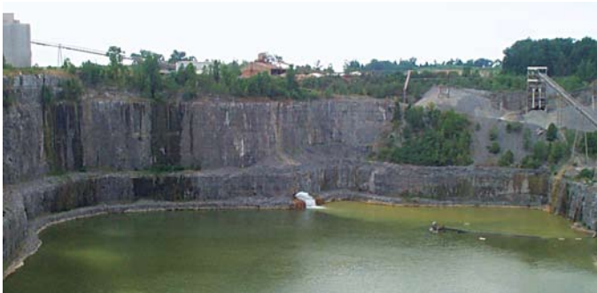
Rooster tail showing a portion of the total 40,000 GPM inflow
