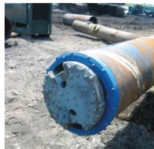
Concentric, shoe-drive, 415Ø, floating crown under-reamer
