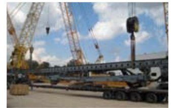
Geo-Foundations' Liebherr LRB 255 torn down and ready for shipping
